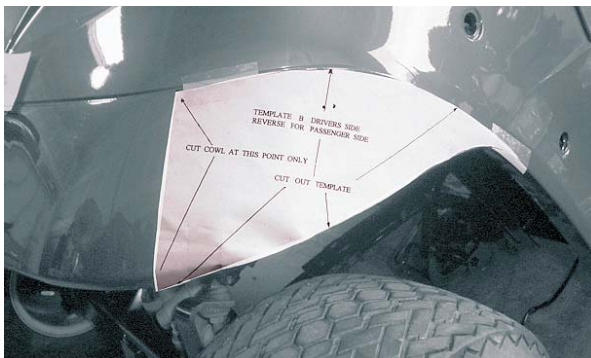
STEP 2: Align template B with body line - Side.
