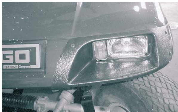
STEP 6: Place headlight assembly along body line and install screws.
